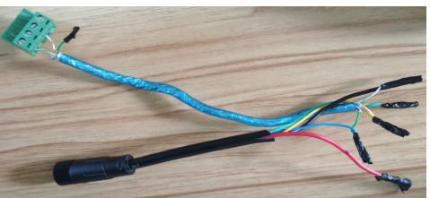
Only connect needed cable when connect female with controller port(No need connect positive wire, Well wrapped with insulation tape), Only connect needed cable when connect network cable with controller port(No need connect green wire, Well wrapped with insulation tape),
