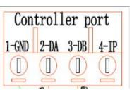
5. Keep male and female connectors tightly fixed between lamps and lamps,Don't reverse connect the signal input and output,Lamp wire core definition is as below:
